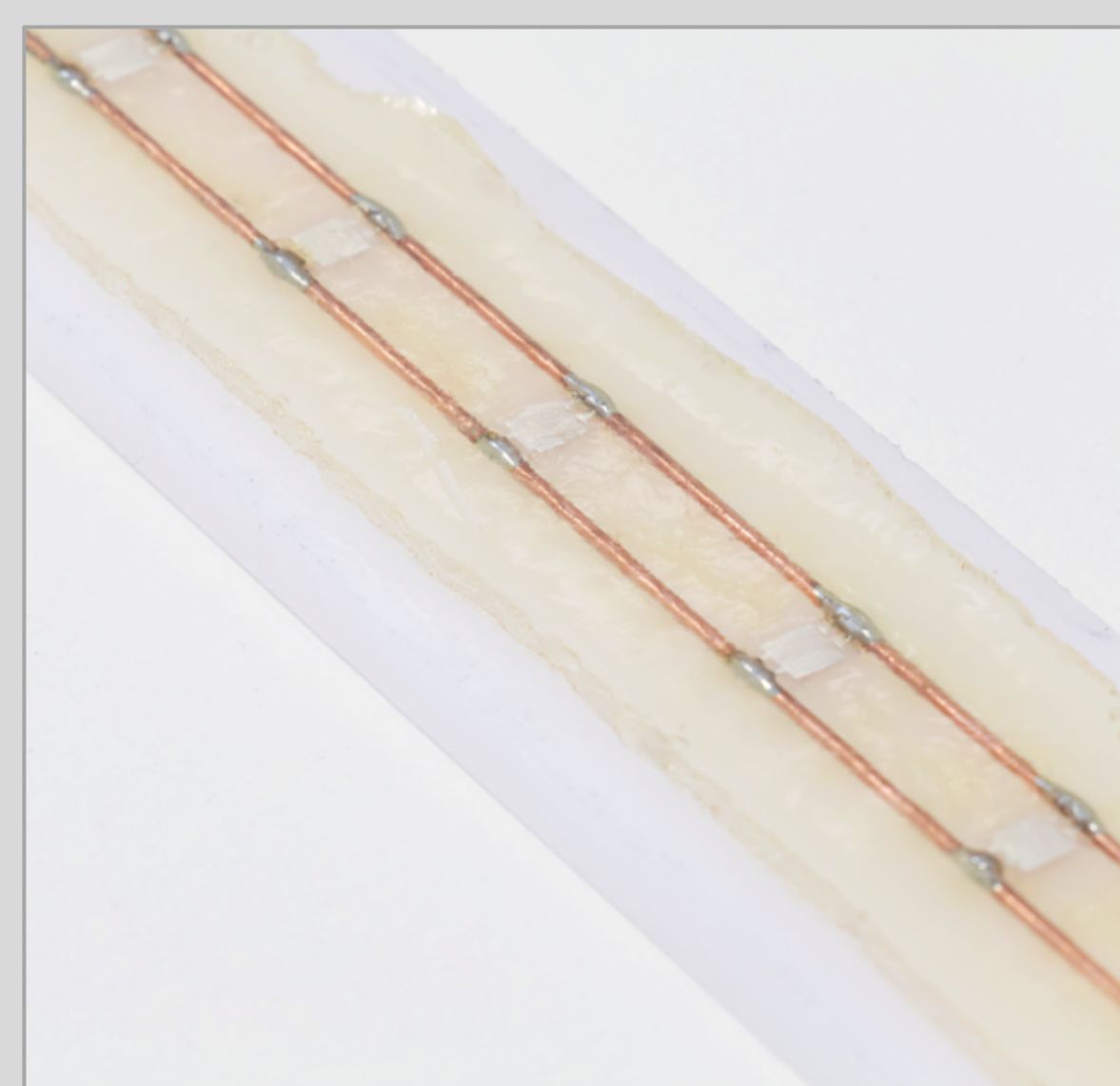
Photodiodes are superglued to an acrylic diffuser bar, soldered to copper wire and sealed in waterproof epoxy.
