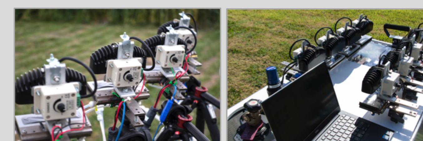
Right – Four of eight custom designed OCTOflux leaf chambers. Left – Control centre of OCTOflux with leaf chambers docked for transport.
