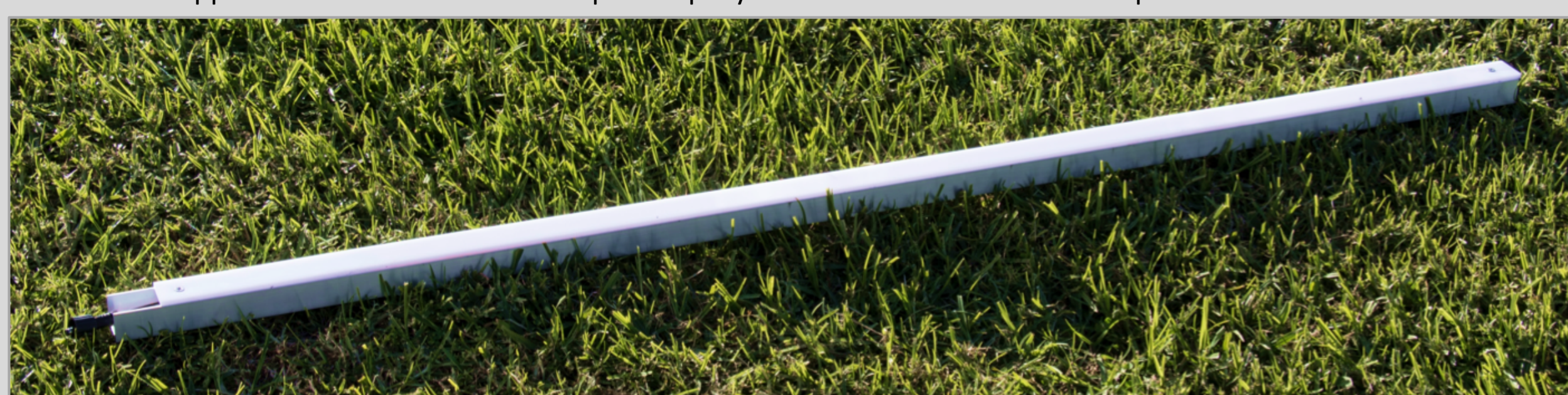
A fully assembled PARbar ceptometer. The acrylic diffuser and photodiodes are mounted on an aluminium channel for rigidity. A waterproof connector is used to connect to the datalogger.
