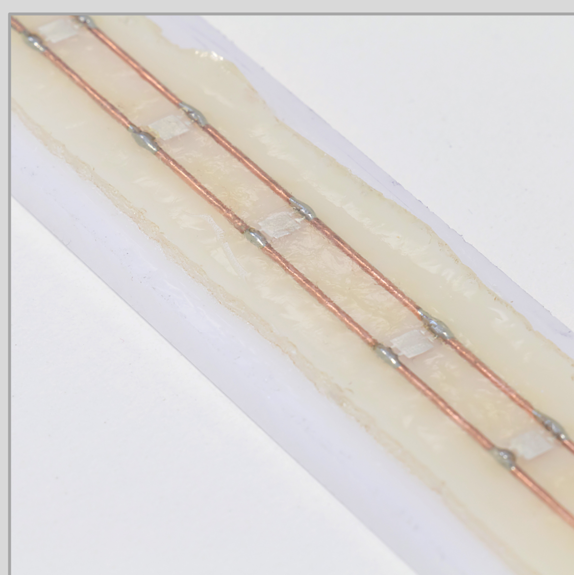
Photodiodes are superglued to an acrylic diffuser bar, soldered to copper wire and sealed in waterproof epoxy.
