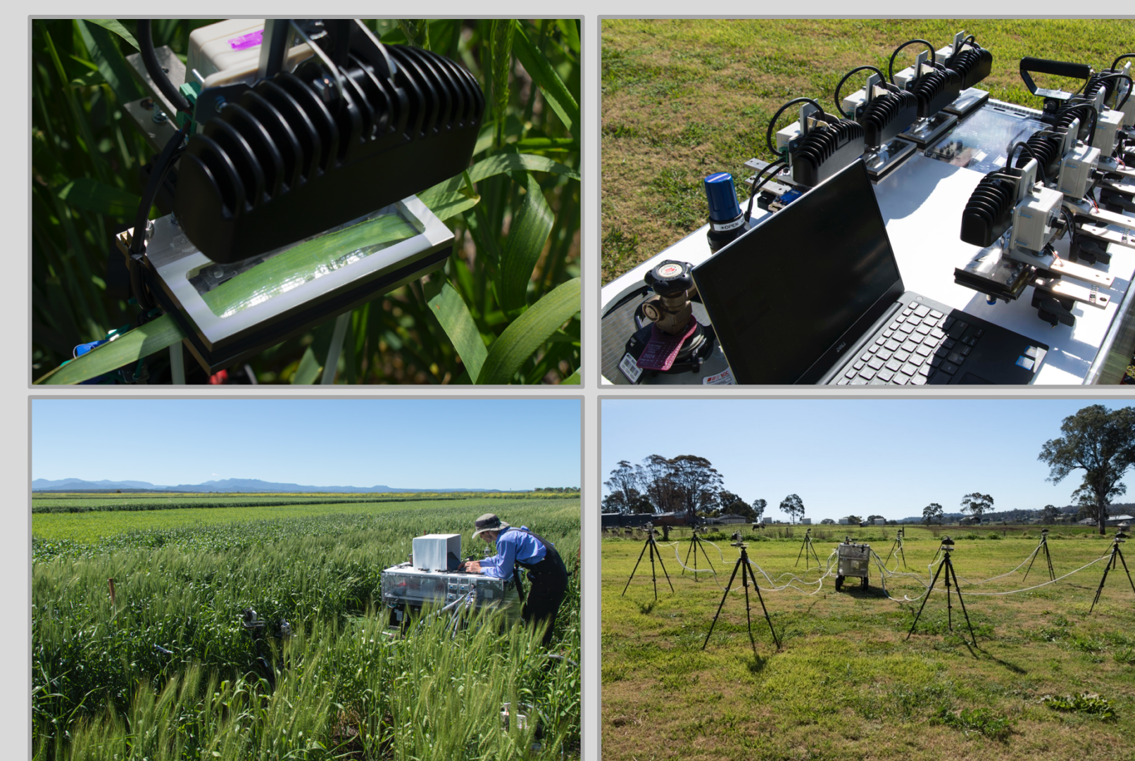
Top right – a wheat leaf in a custom-built OCTOflux leaf chamber with LED light source. Top left – Control centre of OCTOflux with leaf chambers docked for transport. Bottom left – OCTOflux prototype testing in the field in Narrabri, NSW. Bottom right – OCTOflux set up with each leaf chamber on a tripod.
