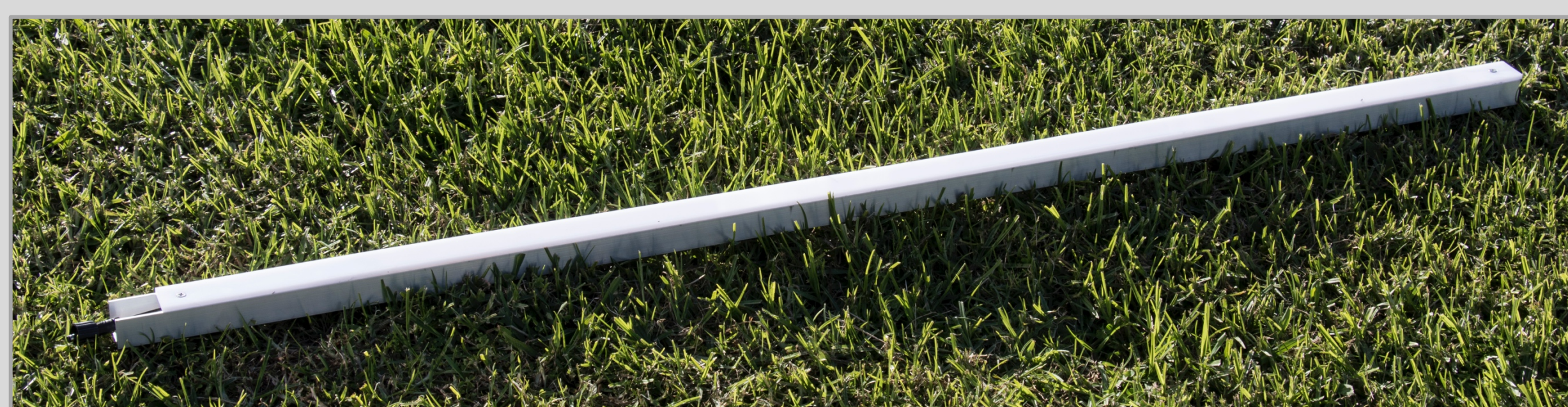
A fully assembled PARbar ceptometer. The acrylic diffuser and photodiodes are mounted on an aluminium channel for rigidity. A waterproof connector is used to connect to the datalogger.
